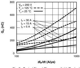
Fig. 7 - Typical Stored Charge vs. dl<sub>F</sub>/dt (Per Leg)
