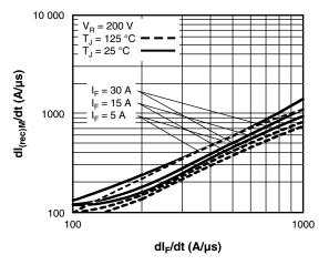
Fig. 8 - Typical dI<sub>(rec)M</sub>/dt vs. dI<sub>F</sub>/dt (Per Leg)
